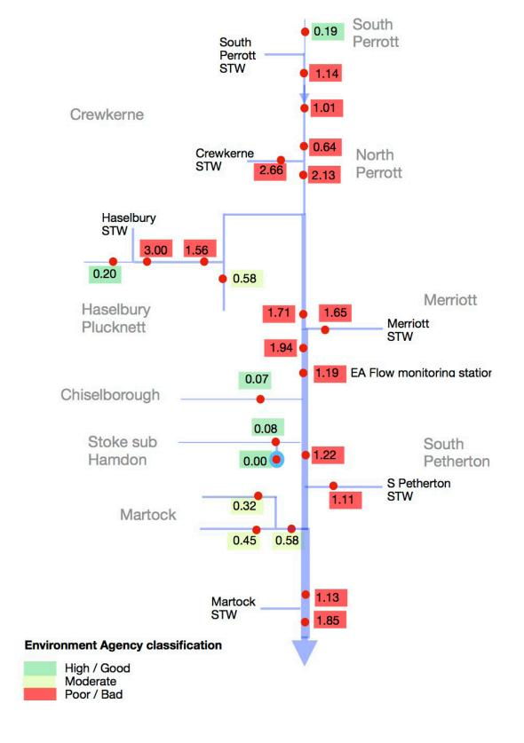
The samples were taken, access permitting, up and downstream of significant confluences. The flow rate was low, about 0.3m3/s at the EA station at Chiselborough bridge. Most of the flow was generated sewage treatment plant effluent. The picture is very similar to that of the survey carried out in the summer of 2022.
